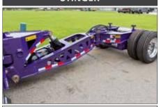
The Stinger Assembly increases the wheel base of the trailer when attached to the rear trailer frame. The Stinger Assembly is used for heavy hauling situations where regulations and specific axle loads must be adhered.
