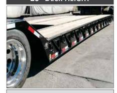
With a standard deck height of 20", Globe Trailers have lower overall height, which allows taller loads to be hauled.
