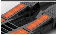
The Air Transition Ramps are recessed in the trailer deck and can quickly be activated to allow loading onto the upper deck.
