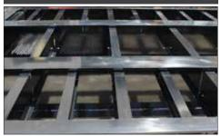
Standard 12" stubbed cross member spacing produces added strength to the trailer and also less stress on the decking, leading to a longer life of the decking material.
