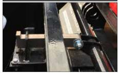
Globe Trailers air lock with safety bar and spring extended pin ensures that the gooseneck locking pin will remain secured even if air pressure is lost.
