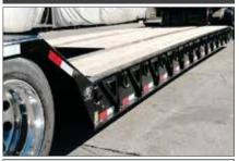
With a standard deck height of 24", Globe Trailers have lower overall height, which allows taller loads to be hauled.
