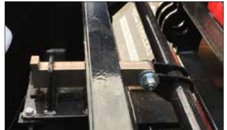
Globe Trailers air lock with safety bar and spring extended pin ensures that the gooseneck locking pin will remain secured even if air pressure is lost.
