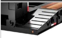
Low profile built-in integrated deck ramps.
