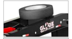
Optional spare tire that mounts securely on top of Gooseneck.
