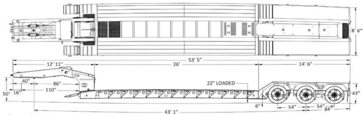
Trailer Model: GTBN553-54-26-HGG Weight: Apx. \_\_\_\_\_ ± lbs
