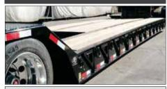
With a standard deck height of 18", Globe Trailers have lower overall height, which allows taller loads to be hauled.
