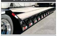
With a standard deck height of 24", Globe Trailers have lower overall height, which allows taller loads to be hauled.
