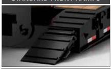
Standard Steel Front ramps, for ease of front loading.
