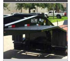
The fenders are in place to help protect the load from flying debris that a truck may create.
