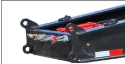
Flip box length options are available to achieve longer swing clearances when needed for longer truck frames or when coupling to single or multi-axle jeeps.
