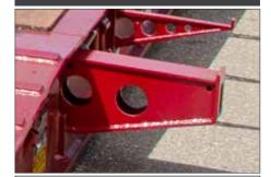
Globe Trailers fabricated heavy duty pullout front outriggers provide added strength which is needed to accommodate the initial force when loading equipment. The outrigger is held in position with a spring loaded locking pin.
