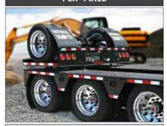
Globe Trailers has a patent on the hydraulic flip axle design. It allows for less down time when operating the flip axle and it can be easily detached when required.
