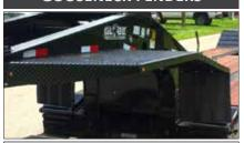
The fenders are in place to help protect the load from flying debris that a truck may create.
