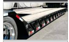
With a standard deck height of 16", Globe Trailers have lower overall height, which allows taller loads to be hauled.
