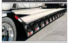
With a standard deck height of 16", Globe Trailers have lower overall height, which allows taller loads to be hauled.
