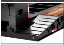
Low profile built-in integrated deck ramps.
