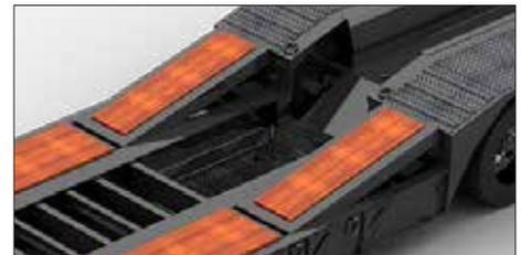
The Air Transition Ramps are recessed in the trailer deck and can quickly be activated to allow loading onto the upper deck.
