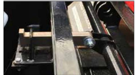
Globe Trailers air lock with safety bar and spring extended pin ensures that the gooseneck locking pin will remain secured even if air pressure is lost.
