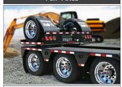
Globe Trailers has a patent on the hydraulic flip axle design. It allows for less down time when operating the flip axle and it can be easily detached when required.
