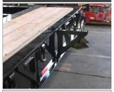
Standard heavy duty outriggers that span the entire height of the side rail allow for maximum force to be applied when in use.
