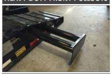
Heavy Duty, dual tubed steel pull out first outrigger.
