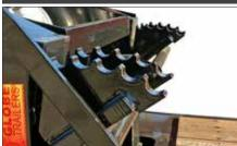
Multi Position Ride Height options. Makes adjustments for various 5th wheel heights easy and allows for larger ground clearance or lower deck height.
