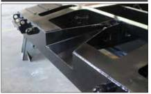
V-Style guide with front tapered beams helps position the gooseneck locking pin, which makes hooking up to a Globe Trailer fast and easy. The locking pin guide rim helps prevent the gooseneck locking pin from coming loose in transit.
