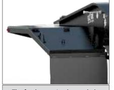
The fenders are in place to help protect the load from flying debris that a truck may create. The left side fenders are provided with acess doors for easy access of gooseneck operation.
