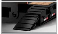
Standard Steel Front ramps, for ease of front loading.
