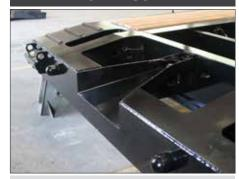
V-Style guide with front tapered beams helps position the gooseneck locking pin, which makes hooking up to a Globe Trailer fast and easy. The locking pin guide rim helps prevent the gooseneck locking pin from coming loose in transit.
