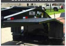
The fenders are in place to help protect the load from flying debris that a truck may create.
