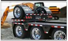
Globe Trailers has a patent on the hydraulic flip axle design. It allows for less down time when operating the flip axle and it can be easily detached when required.
