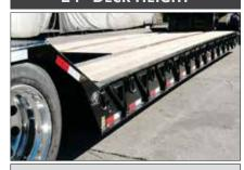
With a standard deck height of 24", Globe Trailers have lower overall height, which allows taller loads to be hauled.
