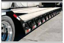
With a standard deck height of 22", Globe Trailers have lower overall height, which allows taller loads to be hauled.
