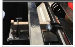
Globe Trailers air lock with safety bar and spring extended pin ensures that the gooseneck locking pin will
