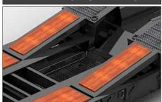
The Air Transition Ramps are recessed in the trailer deck and can quickly be activated to allow loading onto the upper deck.
