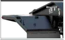
The fenders are in place to help protect the load from flying debris that a truck may create. The left side fenders are provided with acess doors for easy access of gooseneck operation.
