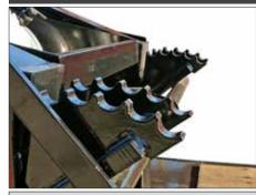
Multi Position Ride Height options. Makes adjustments for various 5th wheel heights easy and allows for larger ground clearance or lower deck height.
