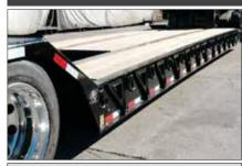
With a standard deck height of 18", Globe Trailers have lower overall height, which allows taller loads to be hauled.
