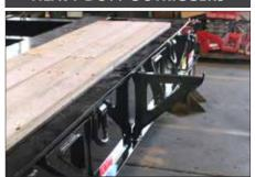
Standard heavy duty outriggers that span the entire height of the side rail allow for maximum force to be applied when in use.
