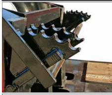
Multi Position Ride Height options. Makes adjustments for various 5th wheel heights easy and allows for larger ground clearance or lower deck height.
