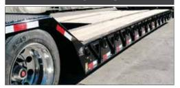
With a standard deck height of 22", Globe Trailers have lower overall height, which allows taller loads to be hauled.
