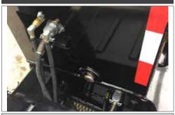
Air, electric and hydraulic (when applicable) fittings are all centrally located at the base of the gooseneck inside a bolster. This makes for quick and easy connect and disconnect. The fittings are protected from possible contact with equipment being loaded or unloaded.
