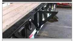
Standard heavy duty outriggers that span the entire height of the side rail allow for maximum force to be applied when in use.
