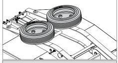
2 Spare tire carriers mounted on top of the Gooseneck
