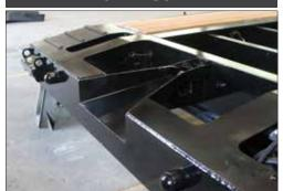
V-Style guide with front tapered beams helps position the gooseneck locking pin, which makes hooking up to a Globe Trailer fast and easy. The locking pin guide rim helps prevent the gooseneck locking pin from coming loose in transit.
