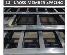
Standard 12" stubbed cross member spacing produces added strength to the trailer and also less stress on the decking, leading to a longer life of the decking material.
