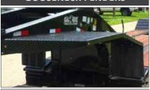
The fenders are in place to help protect the load from flying debris that a truck may create.
