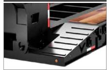
Low profile built-in integrated deck ramps.
