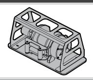
Available options for 20K hydraulic winch system. Mounted front and center of the upper deck. Standard cable length of 85' with shackle. Cable length options are available.
