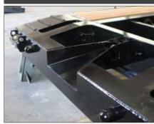
V-Style guide with front tapered beams helps position the gooseneck locking pin, which makes hooking up to a Globe Trailer fast and easy. The locking pin guide rim helps prevent the gooseneck locking pin from
