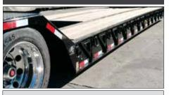
With a standard deck height of 20", Globe Trailers have lower overall height, which allows taller loads to be hauled.
