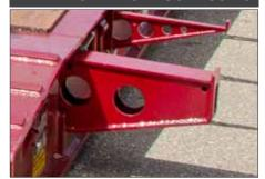
Globe Trailers fabricated heavy duty pullout front outriggers provide added strength which is needed to accommodate the initial force when loading equipment. The outrigger is held in position with a spring loaded locking pin.
