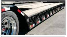
With a standard deck height of 18", Globe Trailers have lower overall height, which allows taller loads to be hauled.
