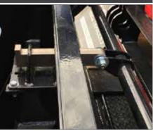
Globe Trailers air lock with safety bar and spring extended pin ensures that the gooseneck locking pin will remain secured even if air pressure is lost.
