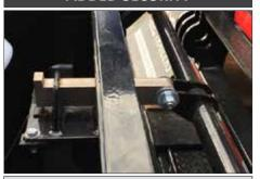
Globe Trailers air lock with safety bar and spring extended pin ensures that the gooseneck locking pin will remain secured even if air pressure is lost.
