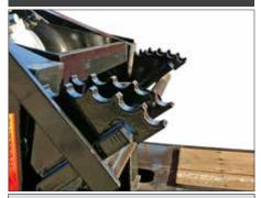
Multi Position Ride Height options. Makes adjustments for various 5th wheel heights easy and allows for larger ground clearance or lower deck height.
