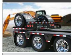
Globe Trailers has a patent on the hydraulic flip axle design. It allows for less down time when operating the flip axle and it can be easily detached when required.
