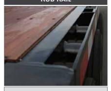
2 ½" rolled formed steel. 6" Structural Channel @ 6.5 lbs/ft, 5/16" Thick Stake Pockets 1 5/8" x 3 ½" x ¼", 24" O/C, ¼" x 3" Rub rail.
