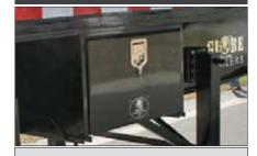
Optional Lockable Tool Box Mounted Underside of Main Deck, 24" x 24" x 48" Steel, can be located on either side.
