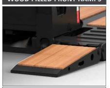
Wood filled, adjustable, spring loaded Low angle paver ramps for easy loading onto the main deck.
