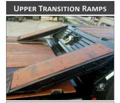
Adjustable sliding transition ramps with wood covering for traction. Ramps are removable.
