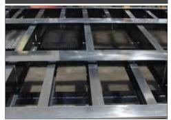
Standard 12" stubbed cross member spacing produces added strength to the trailer and also less stress on the decking, leading to a longer life of the decking material.
